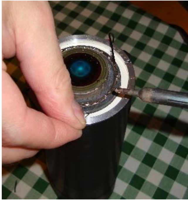
Below is a photo of the negative wire soldered onto the ring.
