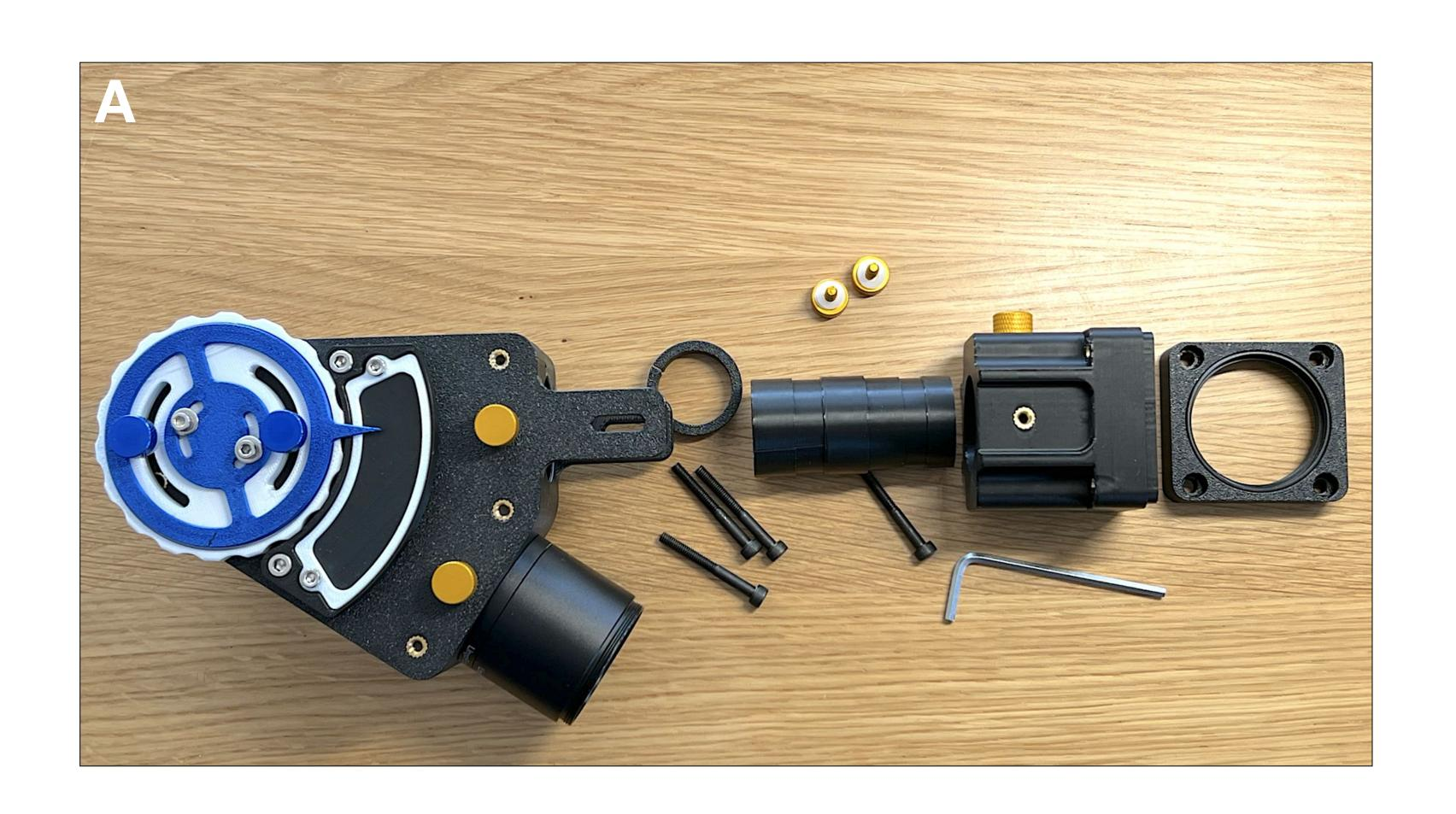
A - Dismantling the collimator + entrance slit system.
