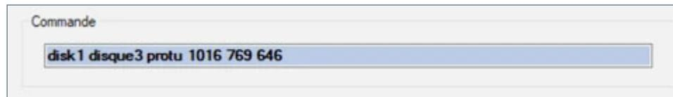
Then type "return". You have surely understood that the numerical parameters are the coordinates of the center of the disc and its radius. If you have any doubts about the syntax of a command, simply type its name and then "Return". You can recall old orders with the up and down arrows, you can modify them, relaunch them by pressing "Return" wherever you are in the edited line ... The i-Spec command line is a "production tool" " very effective.
