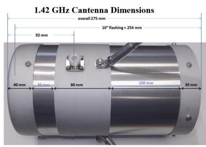
10" wide aluminum flashing (0.010" thick)
